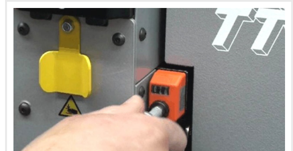
Precise adjustment of the pipe stop.
