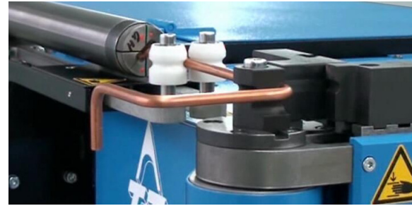
Fully automatic and highly precise bending of pipes up to \varnothing 20 mm.
