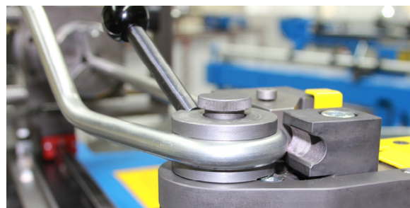
Fast and easy bending of pipe shapes up to Ø 20 mm.
