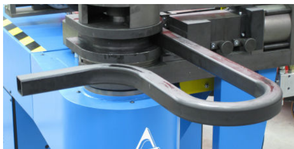
Application example: square steel pipe frame □ 40.0 x 40.0 x 3.0 mm
