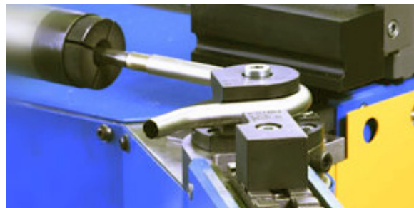
Fully automatic and highly precise bending of pipes up to Ø 20 mm.
