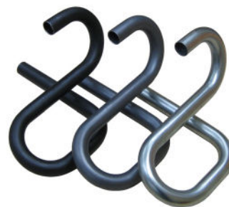
Application example: mild steel pipes Ø 35.0 x 2.0 mm
