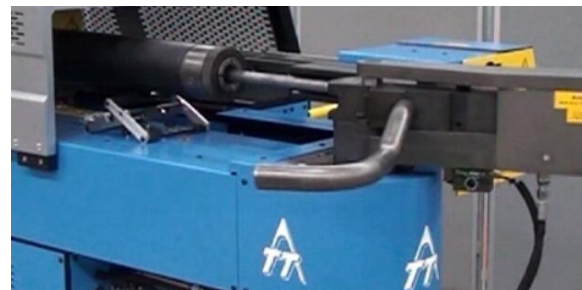
Fully automatic and highly precise bending of pipes up to Ø 60 mm.
